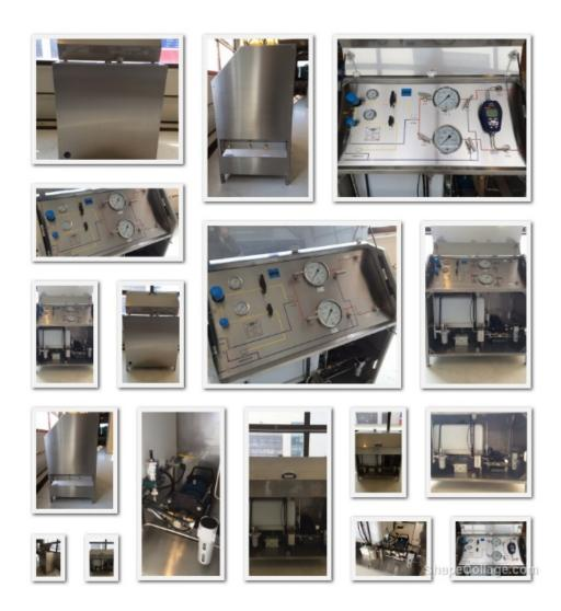
Pressure Test Unit with reservoir. The Unit is built up in a framework of stainless material cowered with panels on all sides. On top of this frame there are mounted a slanted panel where all instruments are mounted. Above this panel, there is a cover with gas dampers. Easy access for forklift / pallet truck.
